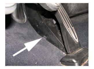
2. Image below shows the accelerator module sliding left after the tab is released. After sliding a short distance to the left, the entire module will lift off.
