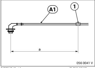
Mark the position of the grommet with adhesive tape (1) on branch **A1**:
