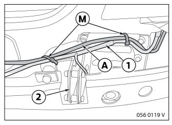
If necessary, secure wiring loom **A** together with **t**he cable for the rear fog lights (1) with cable strap **M** to rear rack mount **AB**.
