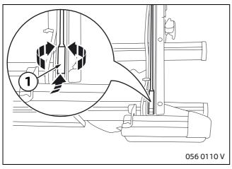
Carefully lift the sliding block (1) out of the guide.
