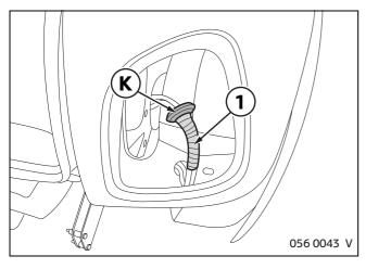
Cut through grommet  $\mathbf{K}$  lengthways and fit around both wiring harnesses at the marking.
