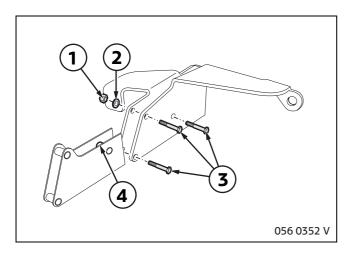
Undo nuts (1) and remove together with washers (2). Remove screws (3) from the mount assy.
