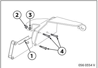
Check bush (1) before starting the work on the two rear rack mounts. If **creme-coloured plastic bushes** (1) are fitted, they must be replaced. For this purpose, order the repair kit, **Part No. 82 71 0 418 155**, and proceed as follows:
