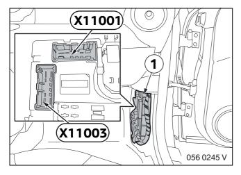
Check at fuse panel (1) whether the contacts are fitted in plug-in slot **X11001** (PIN 9) and in plug-in slot **X11003** (PIN 10). ◀
