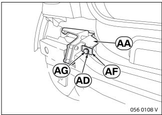
Secure shim **AF** and washer **AD** with screw **AG** through opening (1) to mount **AA**.
