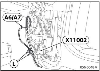
Connect branches **A6** and **A7** with insulation-displacement connector **L** at connector **X11002** of the fuse panel as follows:
