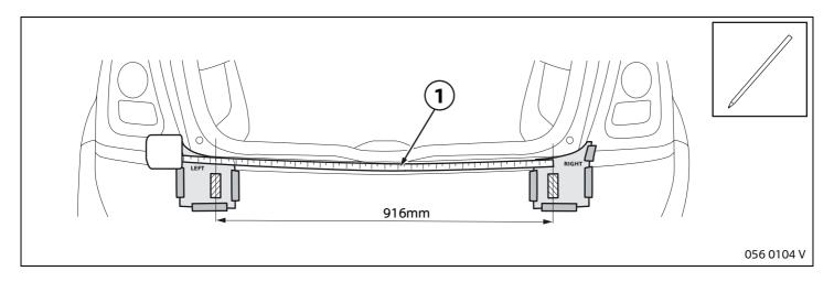
Use a tape measure (1) to transfer the distance between the centres of the templates (= 916 mm, see table on page 7) on to the left-hand side. The distance between centres must be measured along the outer contour of the rear bumper panel.
