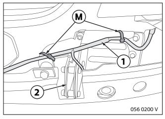
Secure cable for rear fog lights (1) with cable strap **M** to rear rack mount (2).
