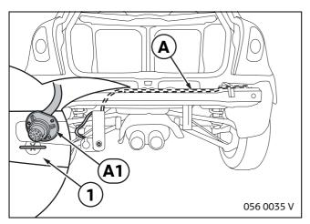
Route wiring loom **A** to the left at the top of the bumper. Pass branch **A1** through the foam material moulding (1).
