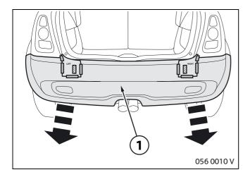
Remove rear bumper panel (1) together with the templates as described under TIS No. 51 12 156.
