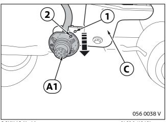
Fit branch A1 in socket bracket C.
