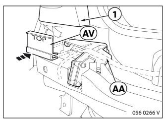
Fit spacing gauge AV on left mount AA.
