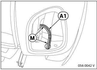
Secure branch **A1** with cable strap **M** to existing wiring harness.
