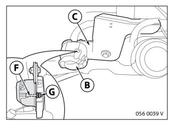
When swivelled upward, it must be possible to open the socket outlet **B** to the right. ◀
