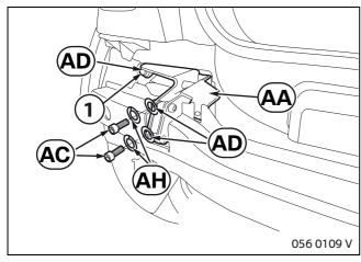
Install left mount **AA** and secure at top left with original screw (1) as well as screws **AC**, washers **AD** a retaining rings **AH**.
