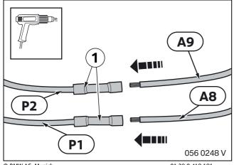
Using connector (1), crimp the insulated branches **A8** (RTVI) and **A9** (RTWS) of the rear rack wiring loom **A** with the branches **P1** and **P2** of the retrofit battery wiring loom **P**.
