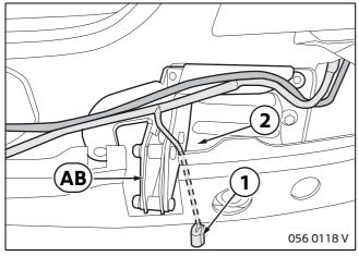
Before securing rear rack mount **AB**, pass the connectors of rear fog lights (1) between rear rack mount **AB** and bumper connection (2).
