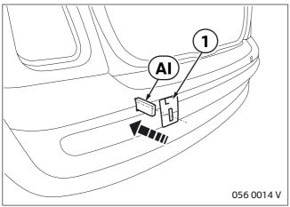
Cut out the matching template (1) (see table on page 7) and slide onto installation tool **AI**.
