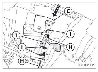
If necessary, remove the sealing compound from the beam and treat the beam with standard MINI corrosion protection measures. ◀
