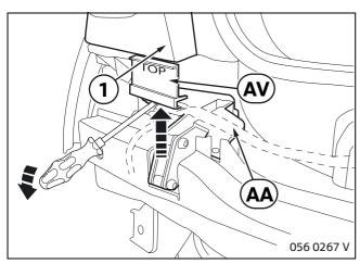
Use a screwdriver to lever up left mount **AA** while screwing down so that the spacing gauge **AV** is clamped free of play between mount **AA** and rear light base (1).
