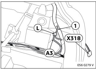
Connect branch **A3** with insulation-displacement connector **L** to wire (GE) of 3rd brake light in vehicle wiring harness (1) as follows:
