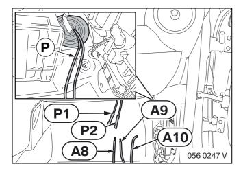
In the vehicle interior, pull cable **P** through the rubber grommet. Seal off the rubber grommet.
