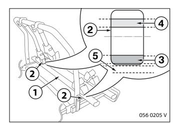
There is a viewing window (2) on both sides under the rear wheel rail (1).
