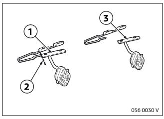
Separate the exhaust bracket (1) at edge (2). Only the separated piece (3) is used for installing the socket bracket **C**.
