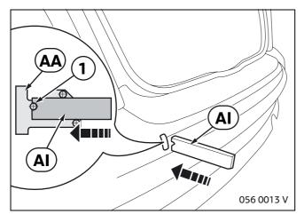
Insert the installation aid **AI** such that the recess (1) is facing upward. The recess (1) must fit on the bearing bush.
