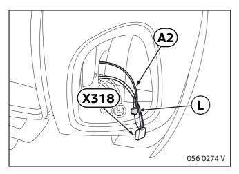
Connect branch A2 with insulation-displacement connector L at connector X318 at right tail light as follows:
