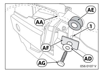
Install spacer bush **AE** between mount **AA** and the crash beam.
