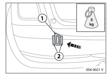
Press the frame (1) against the bumper panel and secure with adhesive tape (2).
