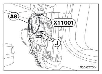
Connect branch **A8**, RTVI wire, at PIN 9 of connector **X11001**.
