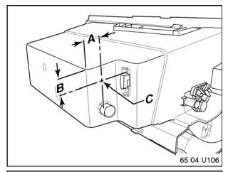
1. Locate and drill 5/8" (16mm) hole in glovebox.
