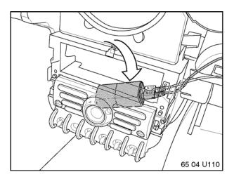
Caution: Check for bent pins on adapter cables before attaching to iPod adapter. If pins are damaged carefully bend them back into position with a small screwdriver.
