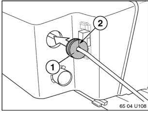
The flat iPod connector (1) should be located in the glovebox and the 8-pin DIN connector (2) for the adapter box should be routed through the center console to a location behind the radio.
