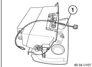
Note: Split grommet as shown before placing around iPod cable in order to prevent damage to cable.
