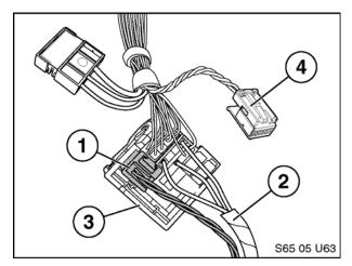
1. Insert pins (1) removed from radio connector into 4-pin connector (2) as follows:
