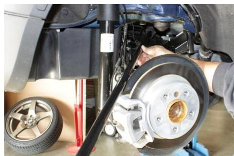
13. Now from right side of vehicle completely remove original bar.
