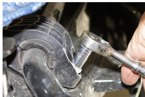
11. Remove the [2] bushing clamp mounting bolts using an E12 Torx or 3/8" socket. Remove clamp. Repeat for other side.
