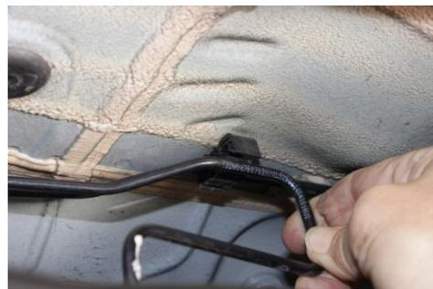
10. **NOTE:** Brake lines will unclip from their support mounts on the uni-body.
