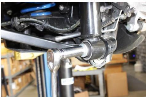
6. Support with jack under trailing arm and remove lower shock absorber bolt using E20 Torx or 5/8" socket. Lower jack to release spring pre-load.
