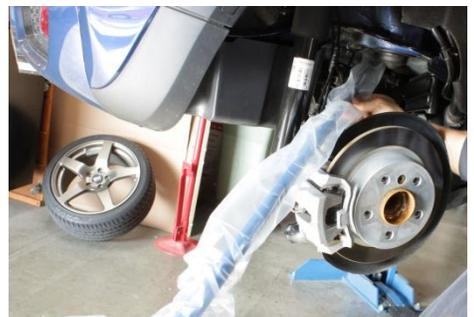
14. Install NM anti-roll bar in reverse of removal of original bar being careful around brake lines. **HINT:** Leave plastic wrap on bar to protect finish of bar during installation through sub-frame then remove.
