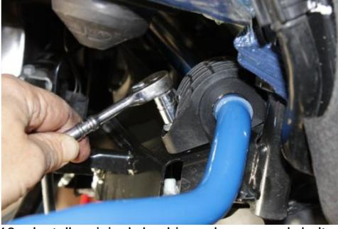
16. Install original bushing clamps and bolts. Torque to 34 Nm (25 ft-lbs).
