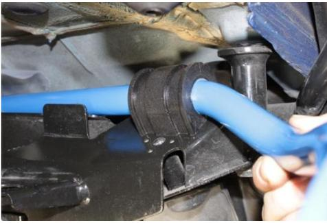
15. Apply supplied grease to inside of supplied urethane bushings and install on NM anti-roll bar.
