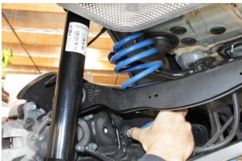
7. Pull down on trailing arm then pull out suspension spring. Repeat steps #6 and 7 for other side.
