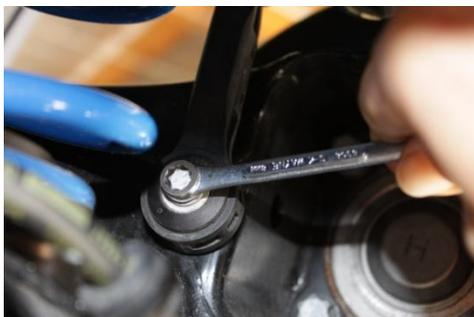
5. Back out lower end-link mounting bolt about a 1/2" using an E10 Torx or 5/16" wrench or socket. Pull down on anti-roll bar arm due to bushing pre-load and then pull out upper end-link stud from bar. Repeat for other side.
