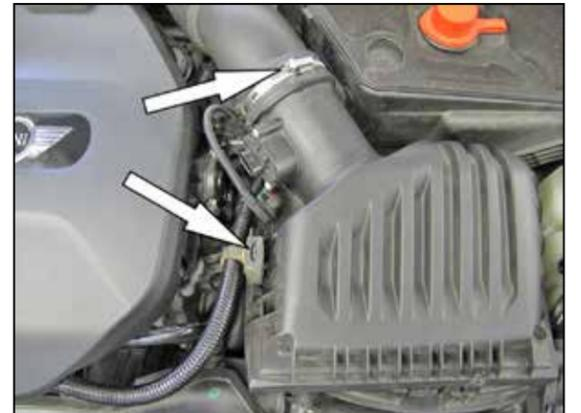
5. Loosen the hose clamp securing the intake tube to the air filter housing and unhook the ground cable from the air filter housing, then lift up the air filter housing and remove it from vehicle.
