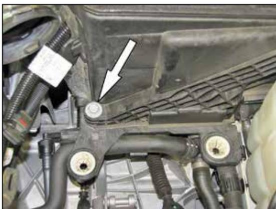
11. Remove the battery cover bolt shown.
