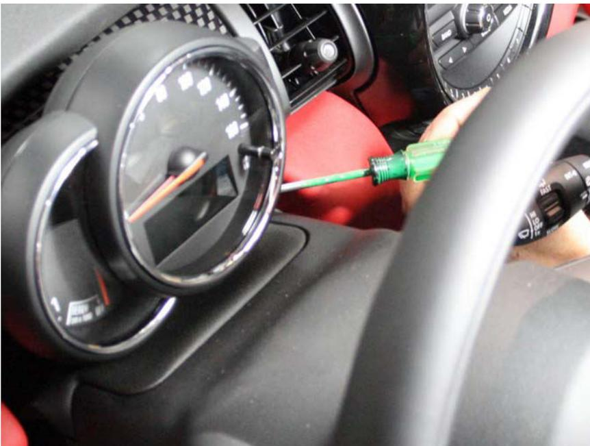
2. Slide the tach towards you and remove the electrical plug from the rear of the tach to free it completely.
