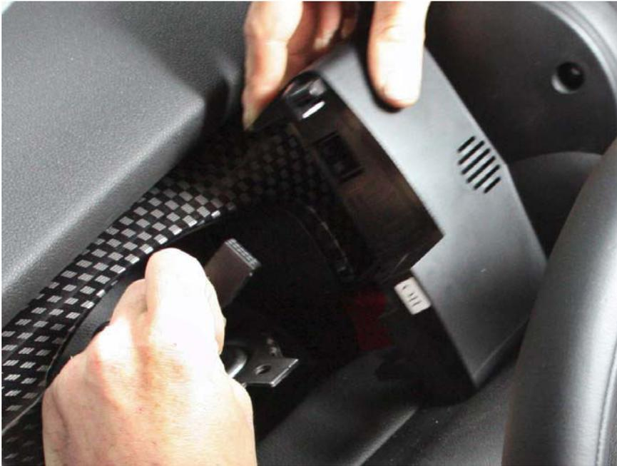
3. Remove the 3 screws (TORX) in the back of the tach.
