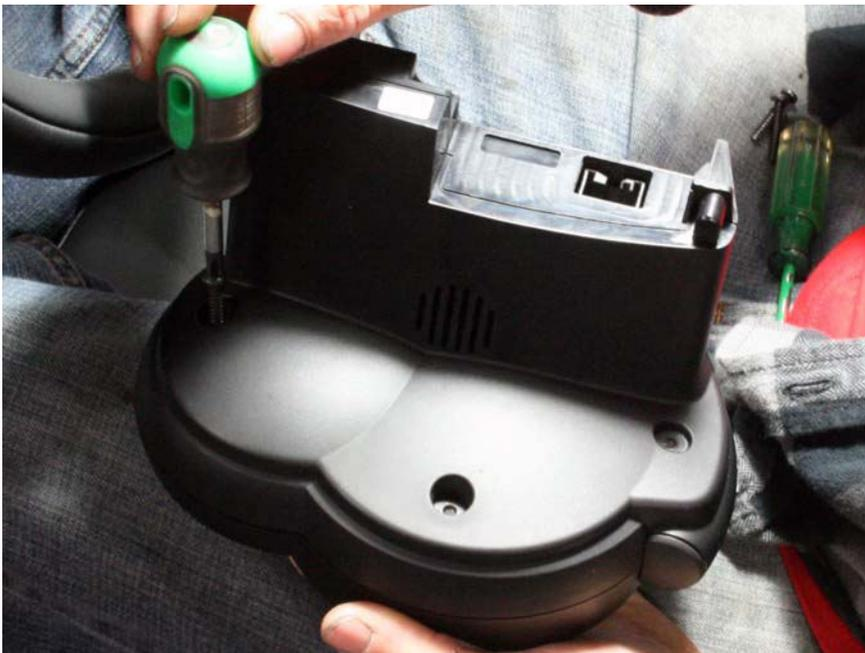
4. Place the “U” bracket in place and using the provided screws, tighten it down.
