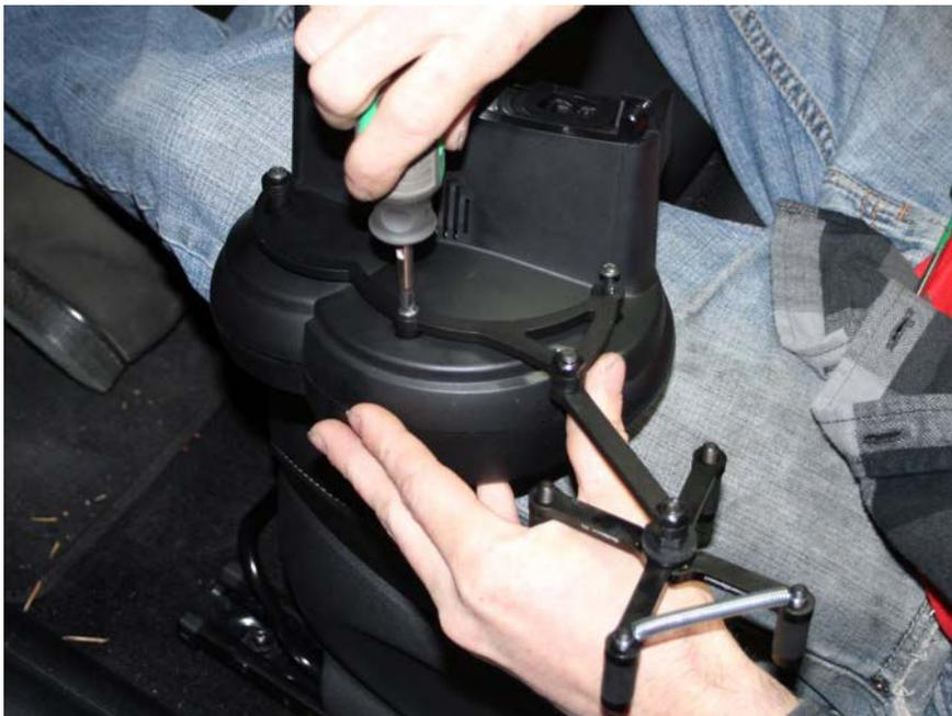
5. Re-connect the electrical clip, slide your tach back into place and put the screws on either side back into place.
