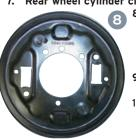
8.Front brake backplate for cars with two wheel cylinders per backplate from 1968 on are made with the adjuster in place. a. For the R/H Backplate ...... 37H2013
