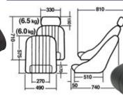
Fixed back traditional bucket seat. A low cost, entry level bucket seat, styled and constructed in a traditional manner. Deep sides and a low back ensure good comfort and support without the restrictions of a larger seat.
