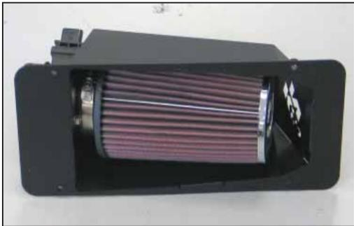
12. Install the K&N® air filter onto the mass air sensor and secure with the provided hose clamp.
