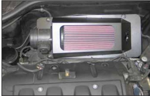
14. Install the heat shield/filter assembly onto the lower air box and secure with the four factory upper air box retaining screws.
