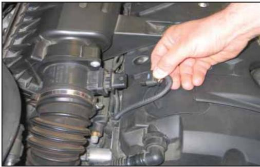
2. Release the locking tab and then disconnect the mass air sensor electrical connection.
