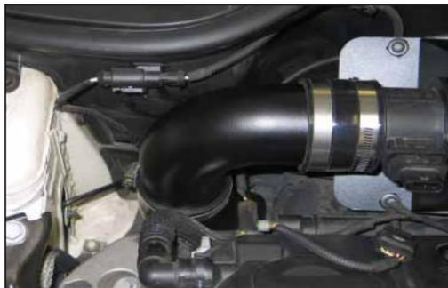
16. Install the K&N® intake tube into the silicone hoses and secure with the provided hose clamps.
