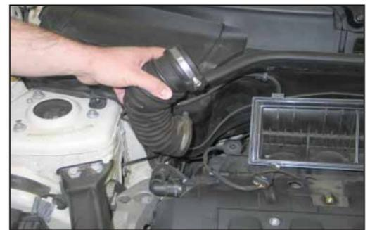
7. Loosen the hose clamp which secures the stock intake hose and then remove the stock intake hose from the vehicle.
