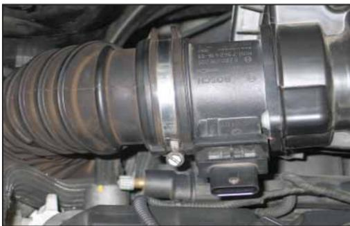
3. Loosen the hose clamp which secures the intake tube to the mass air sensor.
