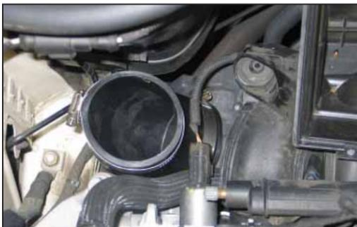
13. Secure the provided silicone hose (08489) onto the throttle body and secure with the provided hose clamp.
