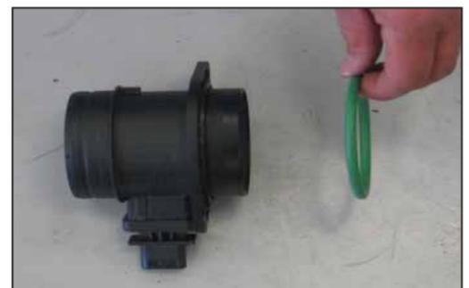
9. Remove the "O" ring from the mass air sensor as shown.
