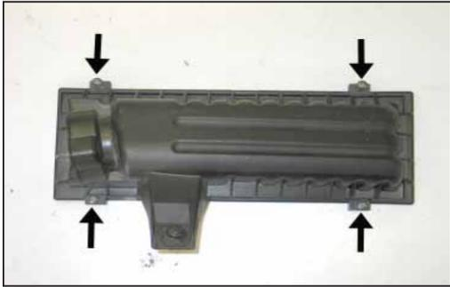
10. Remove the four upper air box retaining screws from the upper air box.
