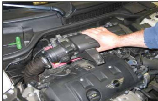
6. Remove the upper air box from the vehicle as shown and then remove the stock air filter.
