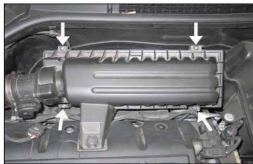
4. Loosen the four screws which secure the upper air box housing to the lower air box housing.
