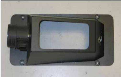
11. Using the provided hardware, secure the factory mass air sensor to the K&N® heat shield as shown.
