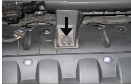
5. Loosen the bolt which secures the upper air box to the valve cover.
