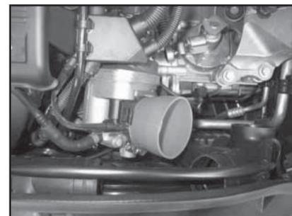
11. Secure the silicone stepped hose & hose clamps onto the throttle body as shown.
