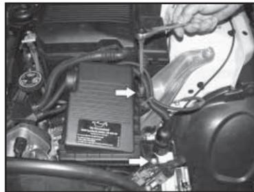
7. Models between April 2001-2004: Remove the two bolts that secure the air cleaner assembly as shown.
