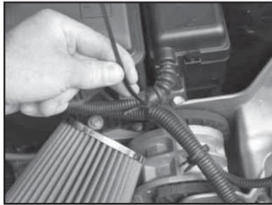
18. Secure the harness away from the air filter using a provided plastic tie as shown.
