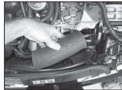
10. Remove the foam feed pipe from between the intake scoop & resonator box as shown.
