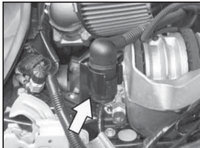
17. Slide the harness multi plug into the bracket as shown.
