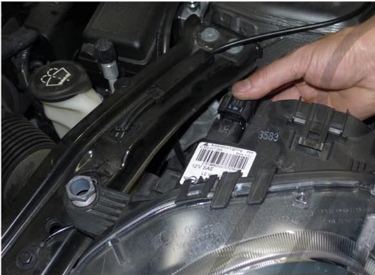
7. Disconnect the headlight harness
