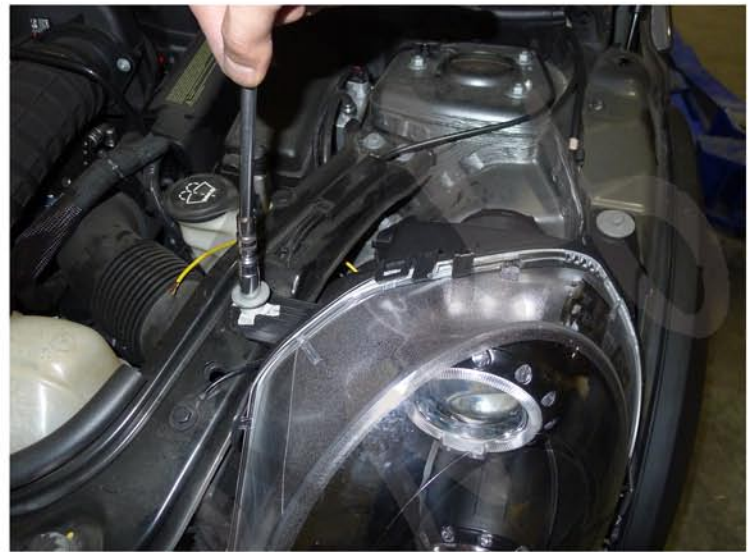
12. Tighten the (2) 10mm bolts
