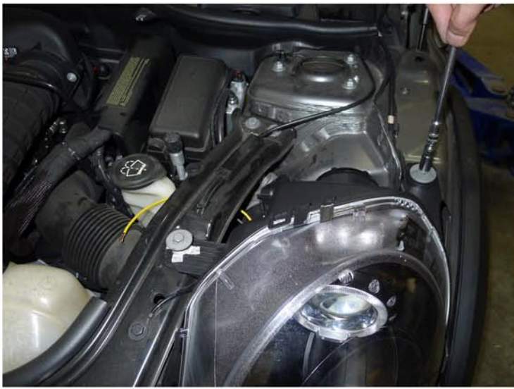
11. Tighten the (2) 10mm bolts
