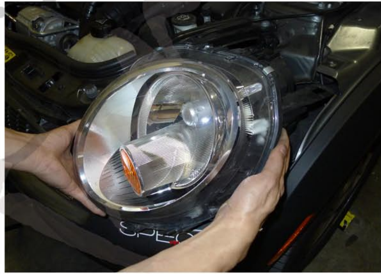
8. Remove the headlight
