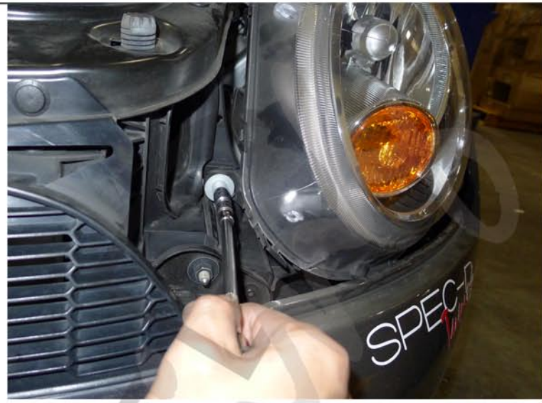
6. Remove the (2) 10mm bolts
