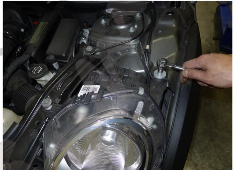
2. Remove the (2) 10mm bolts
