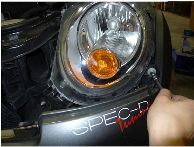
5. Remove the (2) 10mm bolts
