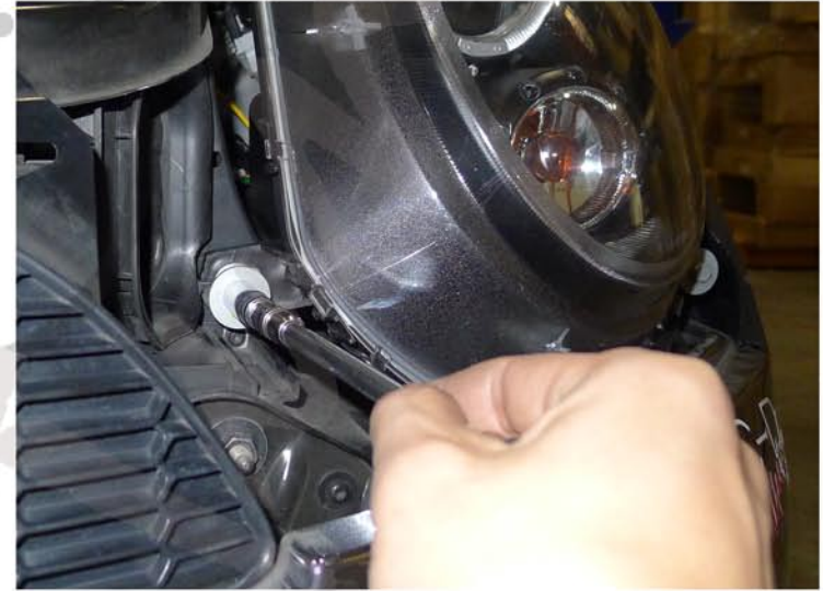
14. Tighten the (2) 10mm bolts
