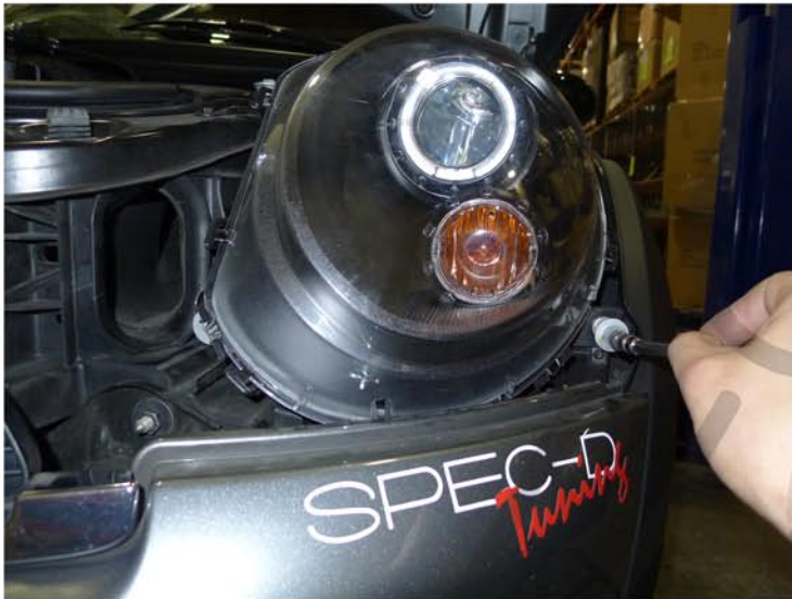
13. Tighten the (2) 10mm bolts
