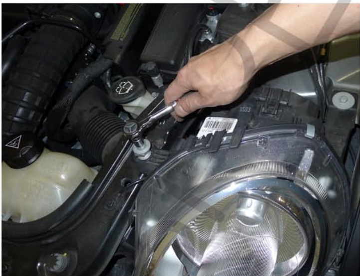
3. Remove the (2) 10mm bolts
