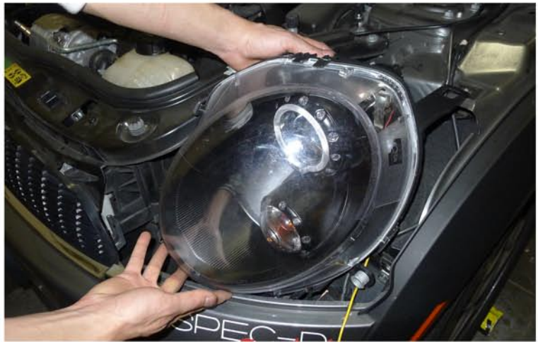
10. Place the new headlight in the stock location
