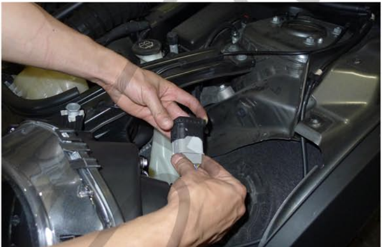
9. Connect the headlight harness to the new headlight Please see the "Halo and L.E.D installation instructions" If your headlights don't have HALO or L.E.D. you can skip it
