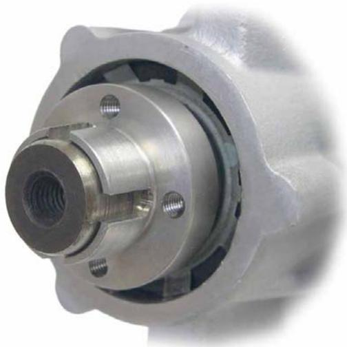
2. Install the pulley with front collar over the rear collar on the shaft. Visually confirm the front collar is fully seated against the end of the shaft.
