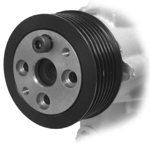
4. Torque each bolt to 72 INCH-Pounds or 5 ft-lbs in a criss-cross pattern, this will take several passes.. Each time a bolt turns, the others will require re-torquing. Continue until all 4 bolts are set to 72 in-lbs or 5 ft-lbs.
