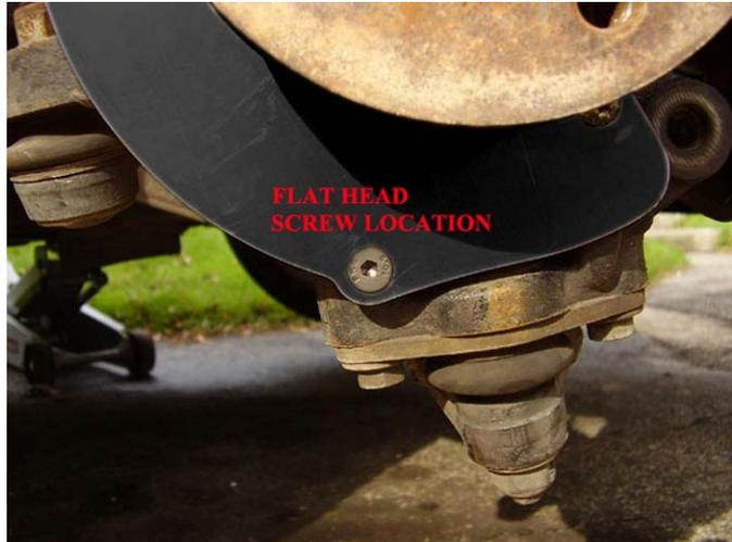
7. Install the scoop on the lower control arm. One method is to position the scoop on the underneath of the control arm and **LOOSELY** secure it with the supplied tie wraps. (You may need to reposition later.)
