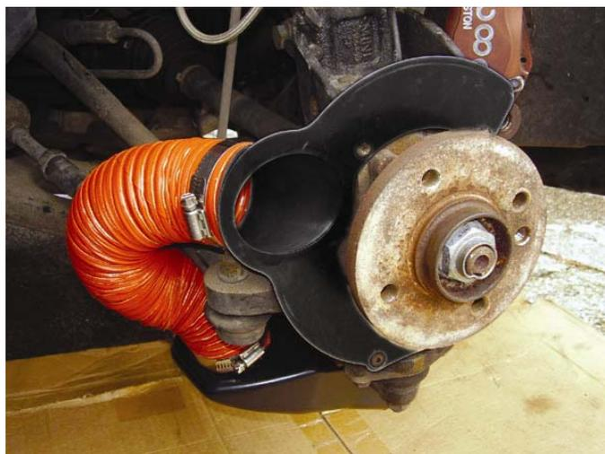
9. Place the rotor back onto the hub.
