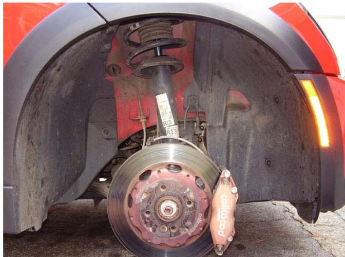
2. Remove the brake calipers by removing the two bolts that secure the calipers to the strut and support them in a way not to damage the brake lines.
