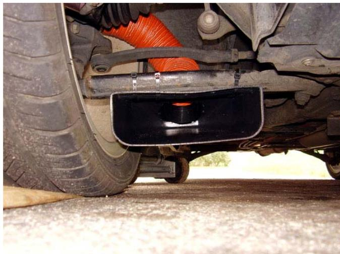
8. Install the hose between the scoop and the backing plate securing at both ends with the supplied hose clamps.
