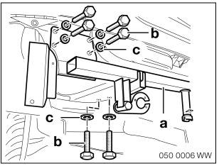
Screw the base part (a) loosely to the left-hand side of the car using screws (b) and washers (c).
