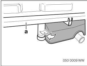
Adjust the heat shield on the exhaust to allow the base part (a) to be mounted on the heat shield.
