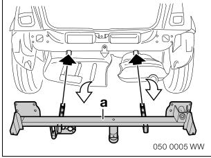
Push the base part (a) with the U-shaped sections into the side members of the car.
