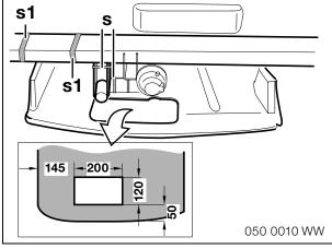
On cars without an emergency wheel the underfloor cover is to be cut out as shown in the drawing.
