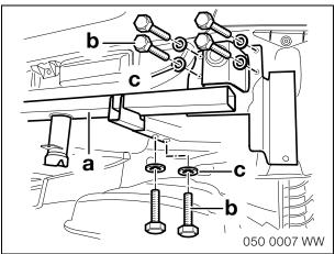
Screw the base part (a) loosely to the right-hand side of the car using screws (b) and washers (c).
