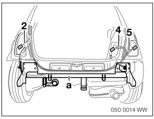
Lay the cable loom (4.5) with 4 plug-in connectors to the right-hand side of the car.
