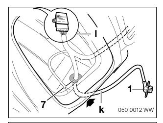
Connect the socket loom on the additional wiring harness (k) from the top through the drilled hole (40 mm in diameter). Fit the passage grommet (7) again.
