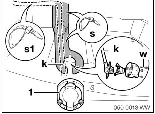
Fit the 13-pin socket (m) as shown. Secure the cable loom with a cable tie (s) on the socket holder and on the base part with a cable tie (s1).
