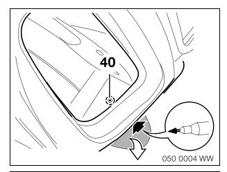
Drill the spot mark below the left tail light to a diameter of 40 mm, deburr it and treat it with anti-corrosion paint.
