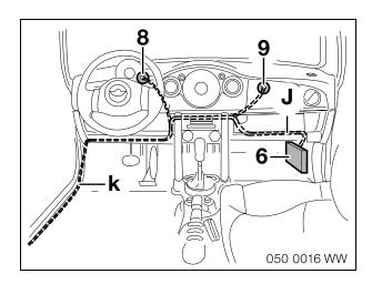
Lay the additional wiring harness (k) along the underside of the dashboard to the centre console and lay the cable (J) on to the light module (6) at the front right using a cable threading coil.
