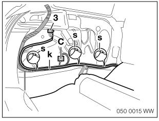
Lay the additional wiring harness (k) as shown along the existing wiring harness to the front to underneath the instrument panel and secure it at suitable points with cable ties (s). Connect the earth connection (C) to the left earth point on the wheel arch.
