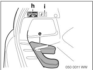
Affix the sticker (h) with details of how to use the ball rod (d) and the nose weight sticker (i) on the rear (degrease the adhesion areas).
