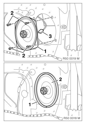
The figure shows the working steps on the left-hand side of the vehicle. The same procedure is to be followed analogously on the right-hand side of the vehicle.
