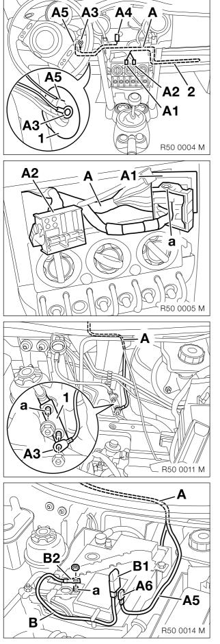
As illustrated, install adapter lead **A** as follows: Route branch **A1** and **A2** to installation location of radio.
