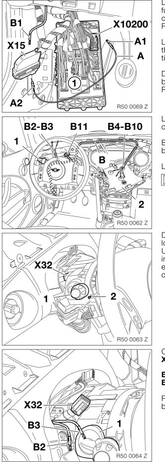
Disconnect the black 12-pin plug **X10200** from the fuse holder II (1) and connect branch **A1**, VI/BR cable, to **PIN 6**. Reconnect plug **X10200** to the fuse holder II (1).
