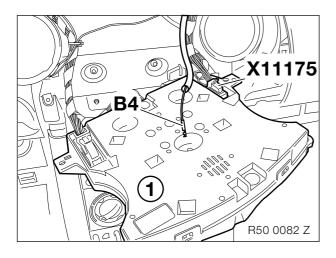
Connect branches B4,~GE/RT cable, to PIN 3 on the black 12-pin plug X11175 .
