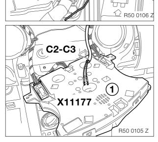
Connect branch **C2**, BL/BR cable, to **PIN 11** on the black 24-pin plug **X11177**.
