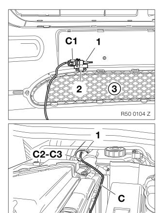
Insert the external temperature sensor (1) into the holder (2) and clip it into the front bumper trim (3) as shown.
