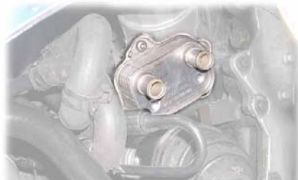
FACTORY OIL COOLER WITH COOLANT LINES REMOVED.
