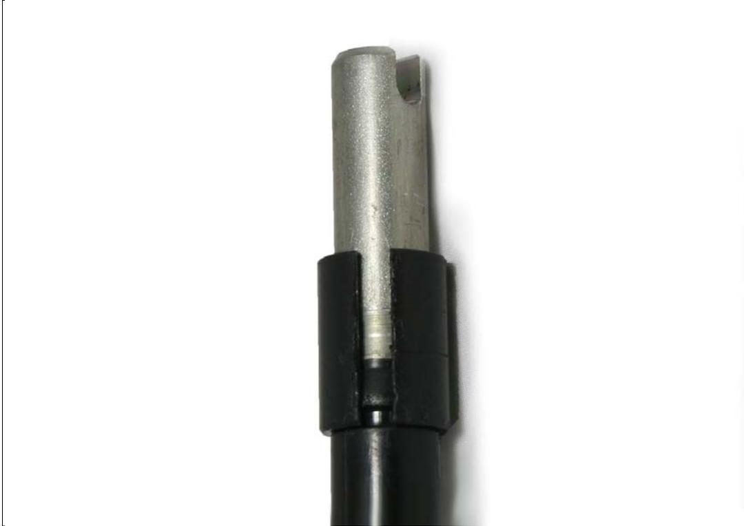
4. Slide Knob Core UP, but not off shifter, around knob core.
