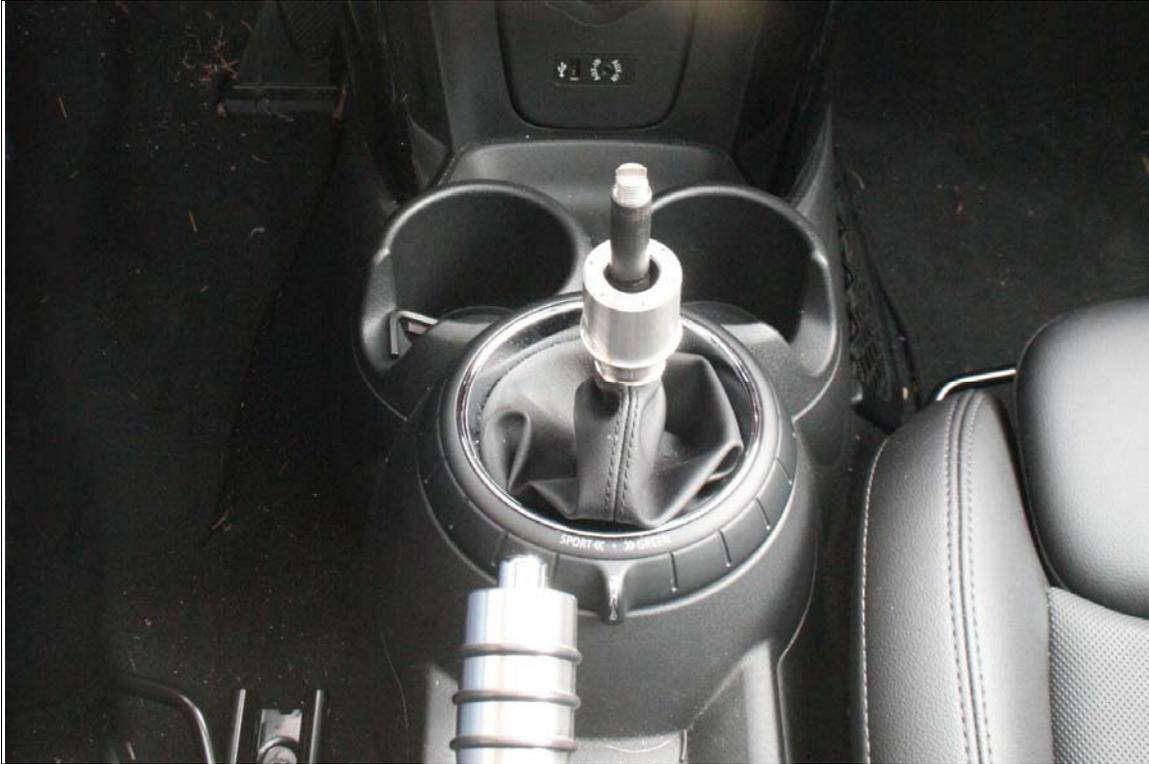
3. Place Knob Adapter over shifter. You'll notice a small collar on one end of the adapter, that collar will be facing DOWN, when you slide it over the shifter, it will click into the indented section (Seen below).
