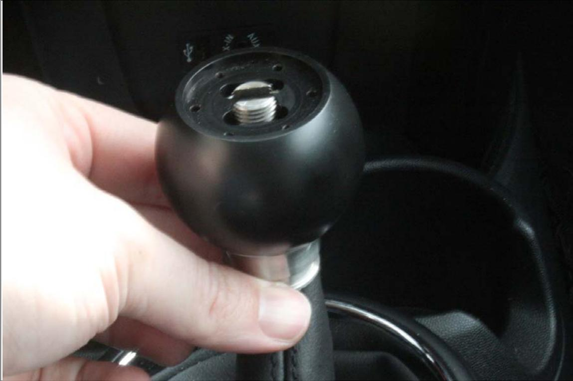
7. Place cap on your new knob, and install the 6 (2mm Hex) screws.
